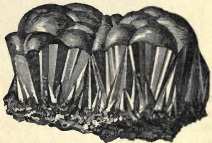
FIG. 64.—Piece of hæmatite, showing the nodular external form and the internal crystalline structure.
